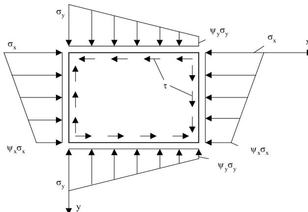
Fig. 3.6.7.3. Plate subjected to combined in-plane load
