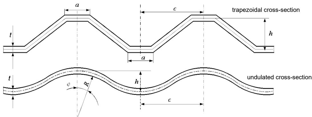
Fig. 4.5.1. Trapezoidal and undulated cross-sections
