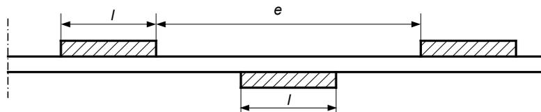
Fig. 2.2.3.2-2. Staggered welds
