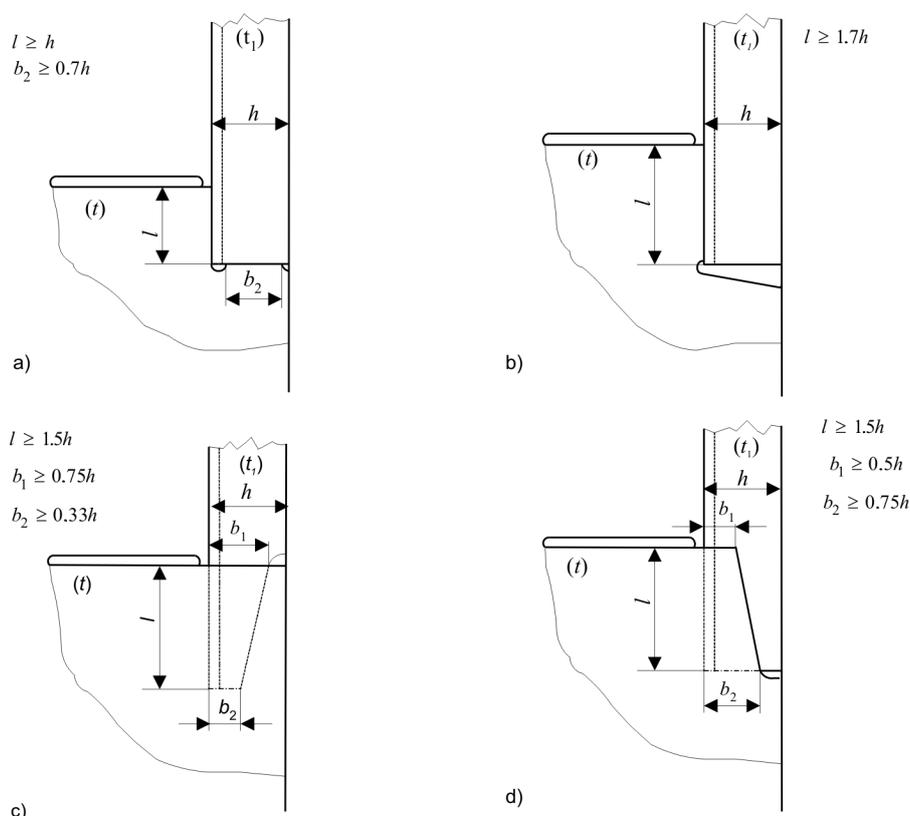
Fig. 4.3.4. Required design patterns for connection of stiffener ends to girders or brackets
