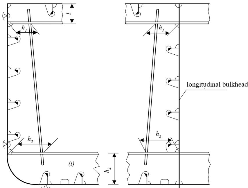
Fig. 7.4.3.8. Construction of framework in frame planes with bottom floors applied
