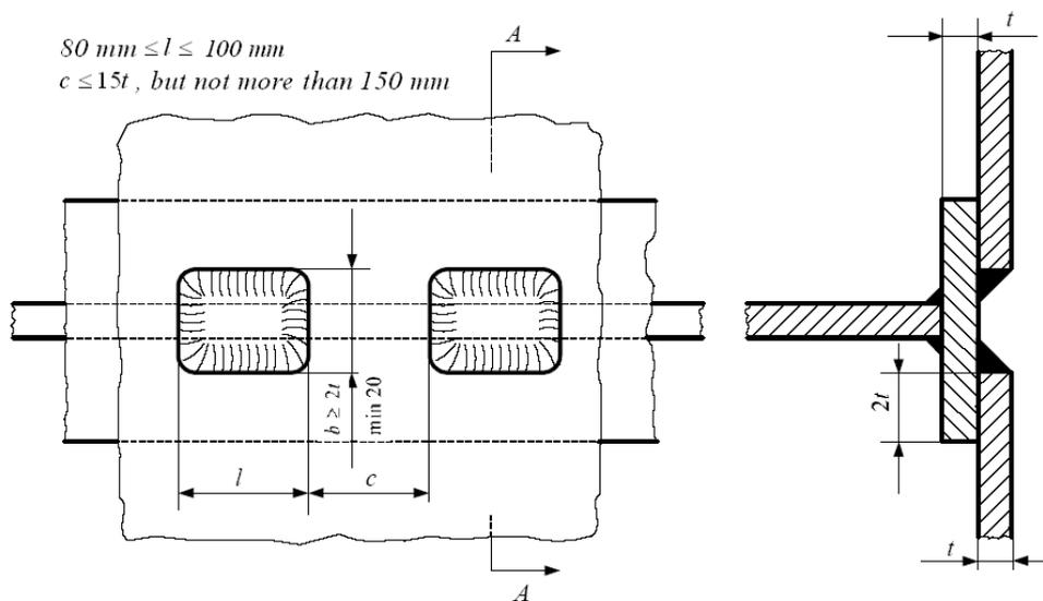
Fig. 2.2.5.1-2. Slot weld with backing
