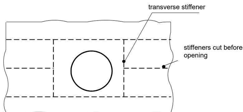
Fig. 4.4.4. Stiffening of plating in way of opening
