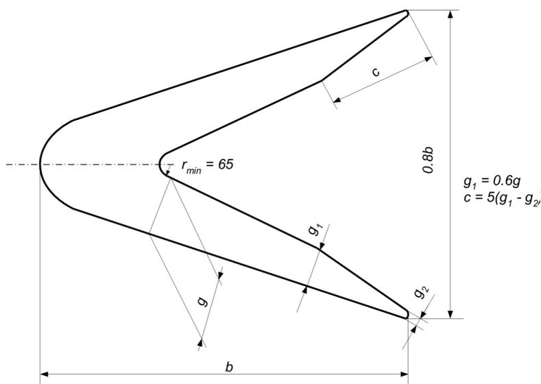
Fig. 5.8.7.3. Cross-section dimensions of propeller post
