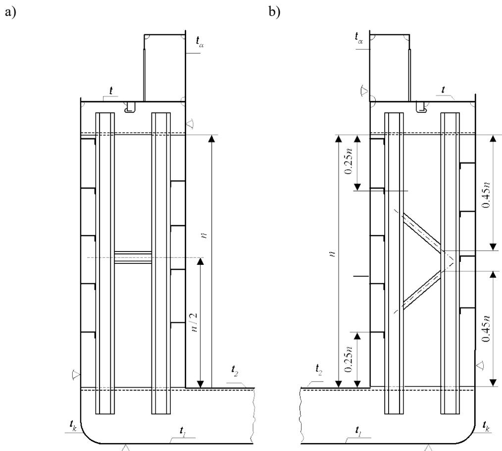
Fig. 7.1.1.1. Typical stiffening system in double-hull barges
