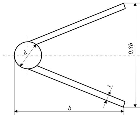
Fig. 5.8.7.6. Propeller post with round bar construction
