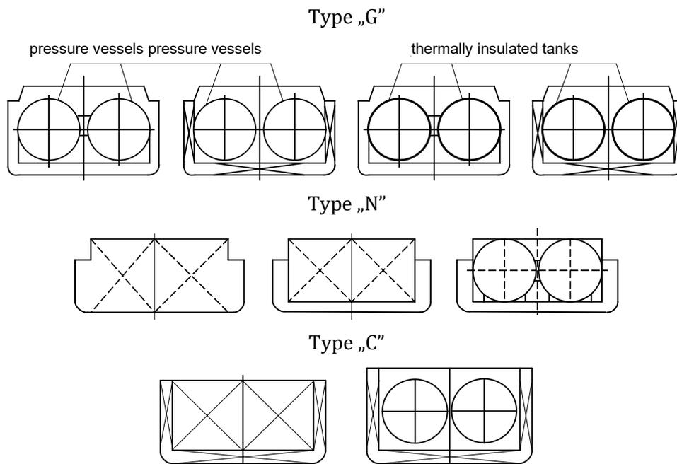
Fig. 7.12.2.1. Types of tankers for carriage of hazardous cargoes
