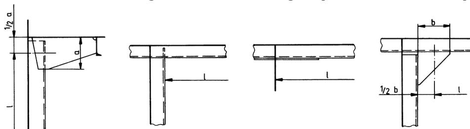
Fig. 3.4.2.4. Stiffener span determination pattern
