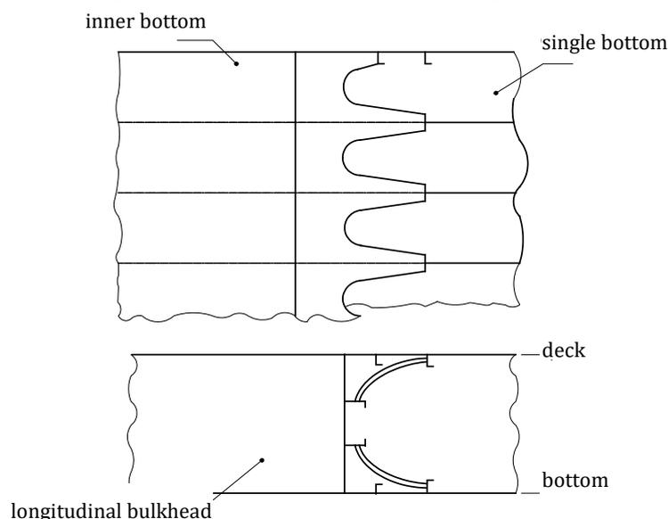
Fig. 4.2.7. Recommended design patterns for reduction of stress concentration
