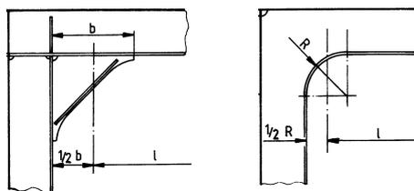
Fig. 3.4.3.2. Girder span determination pattern
