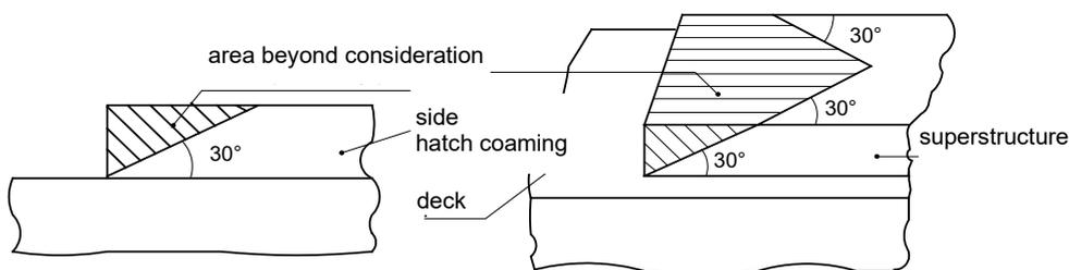
Fig. 3.3.2.3-1. Principle of consideration of hatch side coamings and superstructures
