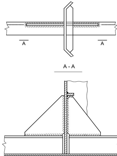
Fig. 4.5.4. Fixing of plating stiffeners to corrugated bulkhead
