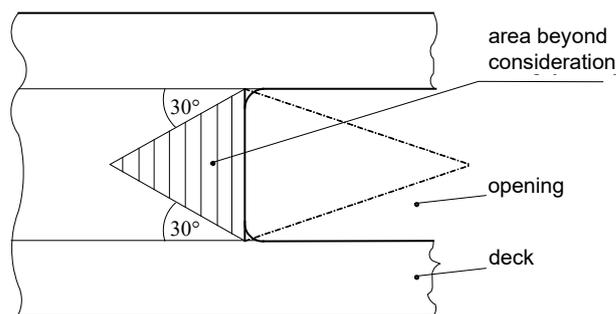
Fig. 3.3.2.2-1. Principle of consideration of deck openings
