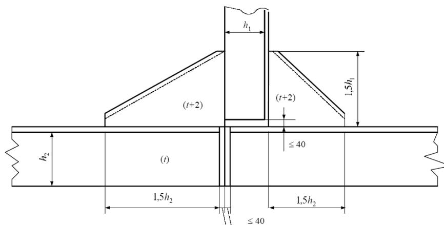
Fig. 7.4.3.5. Recommended construction of bottom longitudinal connection to bulkhead
