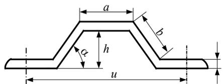
Fig. 5.7.8.2. Scantlings of corrugated bulkhead member with trapezoidal cross-section
