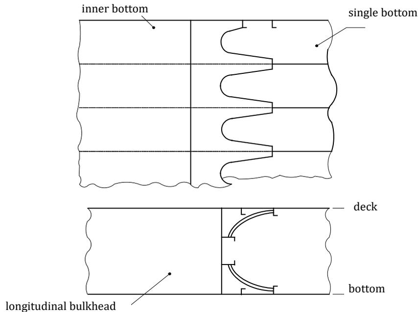
Fig. 2.7.2.7 Recommended design patterns for reduction of stress concentration
