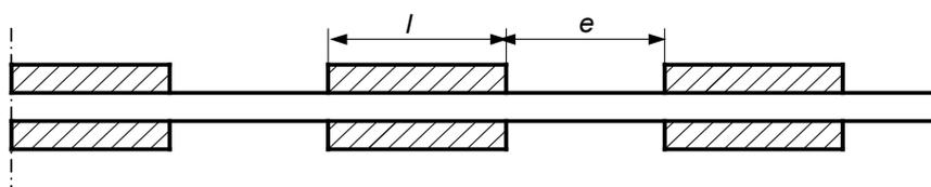
Fig. 2.3.2.3.2-1 Chain welds
