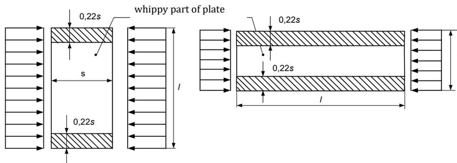
a) transverse framing system ( $s/l \leq \sqrt{2}$ ) b) longitudinal framing system ( $l/s > \sqrt{2}$ )
