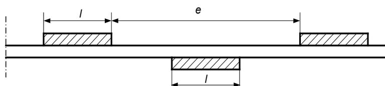
Fig. 2.3.2.3.2-2 Staggered welds
