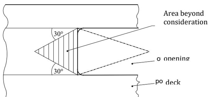
Fig. 2.5.4.2.2 Principle of consideration of deck openings
