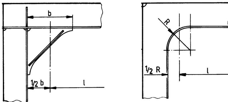
Fig. 2.5.5.3.1 Girder span determination pattern
