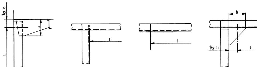
Fig. 2.5.5.2.4 Stiffener span determination pattern
