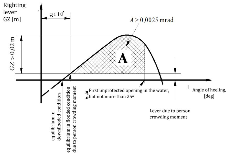
Fig. 3.1.2 Righting lever curve
