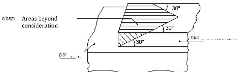
Fig. 2.5.4.2.3 Principle of consideration of longitudinal structure members in way of their ends
