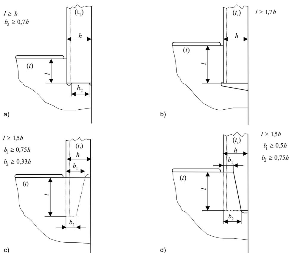
Fig. 2.7.3.3 Required design patterns for connection of stiffener ends to girders or brackets
