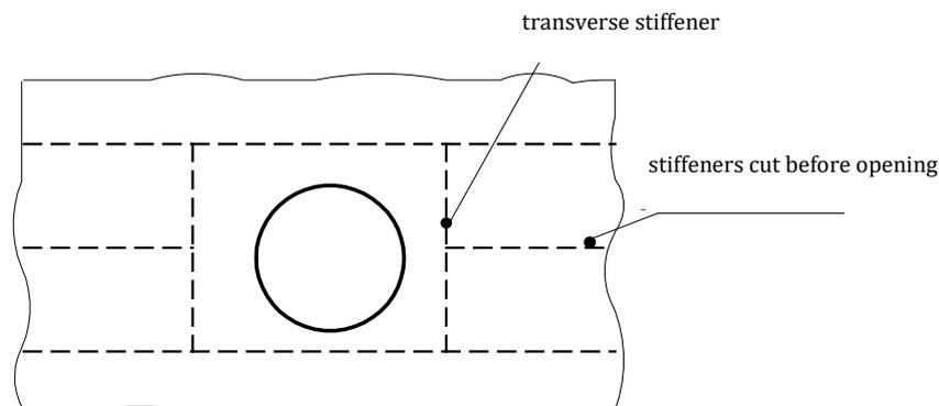
Fig. 2.7.4.4. Stiffening of plating in way of opening
