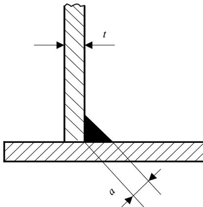
Fig. 2.3.2.3.3 Thickness of weld  $a$
