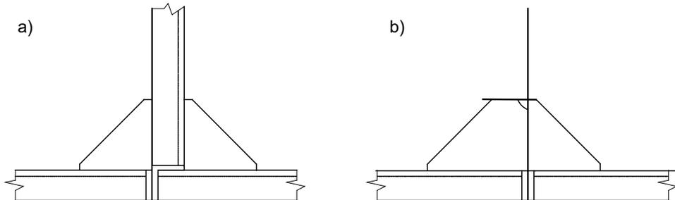
Fig. 2.7.3.7. Recommended design patterns for connections of stiffeners to girders, divisions or bulkheads
