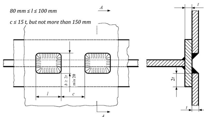
Fig. 2.3.2.5.1-2 Slot weld with backing
