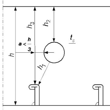
Fig. 2.5.5.3.4 Determining of web net height
