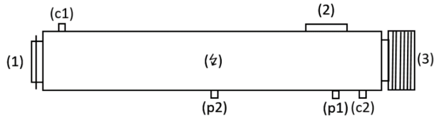
Figure 3 Configuration with ERD (3) mounted at the front end of the test vessel
