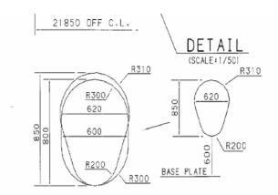
3. If a vertical opening is at a height of more than 600 mm, steps and handgrips are to be provided. In such arrangements it is to be demonstrated that an injured person can be easily evacuated. (IACS UI MODU 1) and (MSC.1/Circ.1544)
