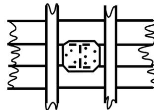
Joint by steel butt strap
