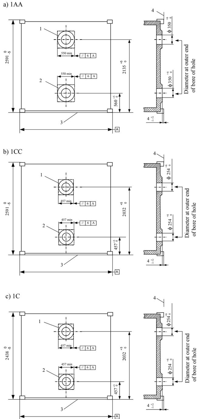
Fig. 2.7.2. Ventilation openings in the end wall of 1AA, 1CC and 1C containers
