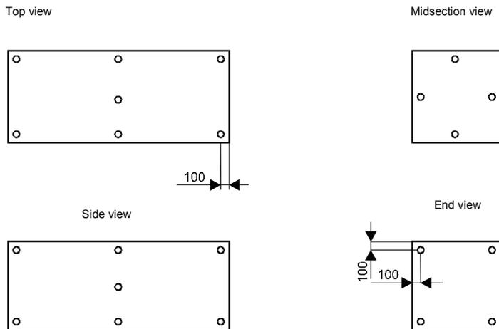
Fig. 3.5.3-1. Air temperature measurement points inside the container
