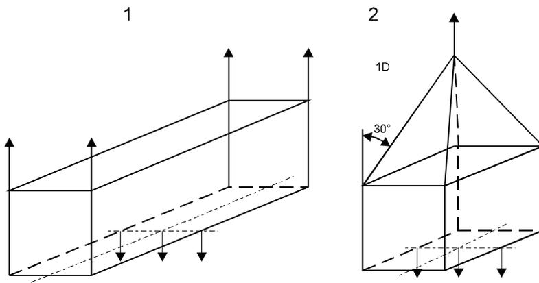
Fig. 3.2.2.3. Lifting from the top corner fittings
