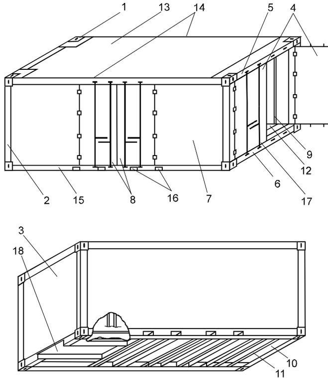
Fig. 1.2. Structural elements of a container (general purpose)
