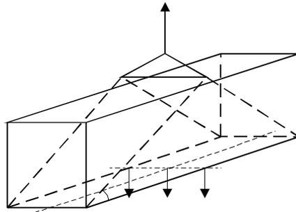
Fig. 3.2.2.4. Lifting from the bottom corner fittings
