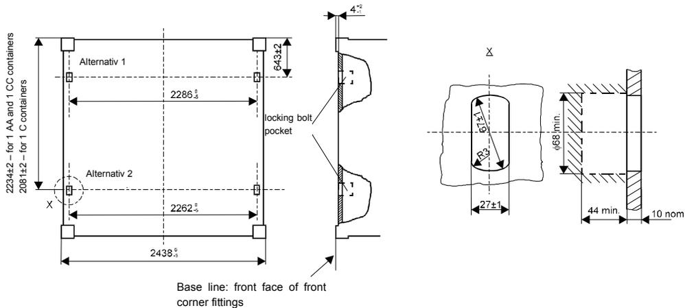
Fig. 2.9. Arrangement of intermediate sockets for clip-on units
