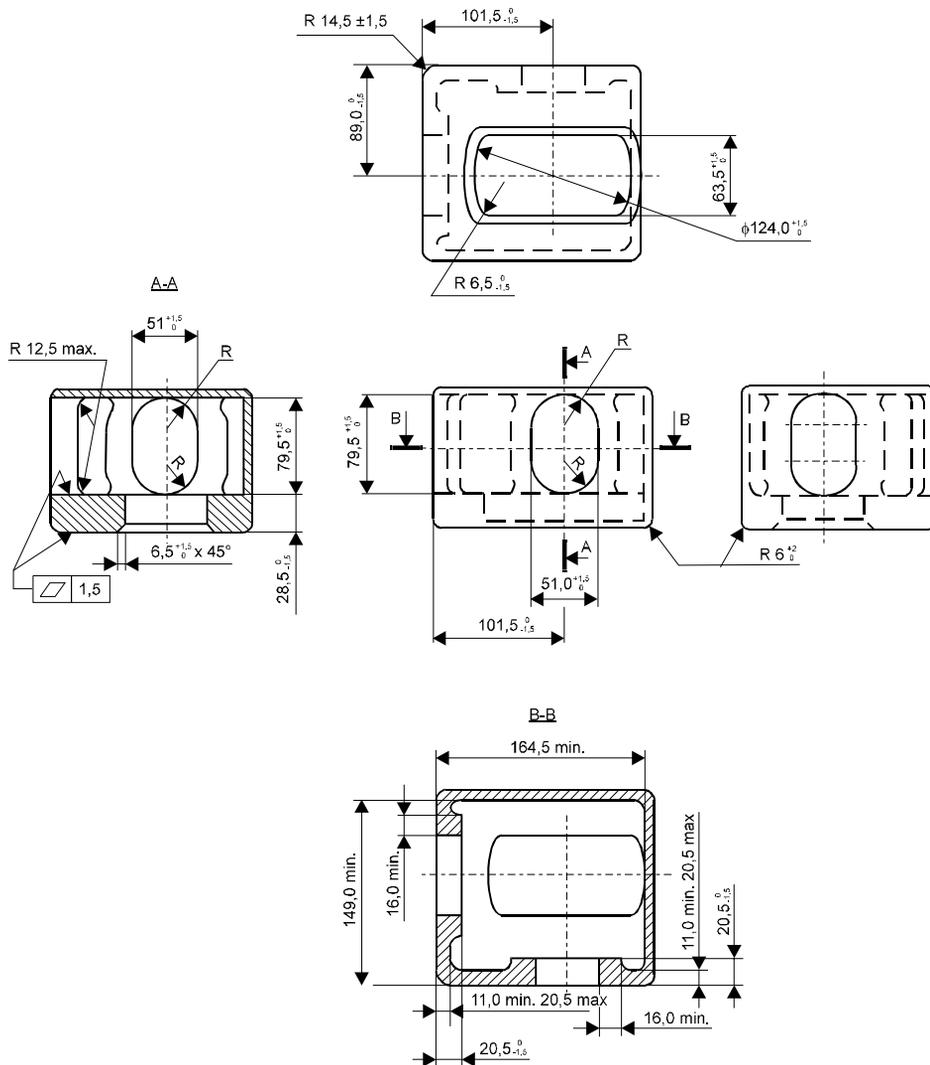
Fig. 3.2.1.1-3. Bottom corner fitting
