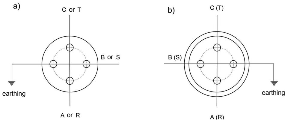
Fig. 2.11.3.4. Phase-sequences on the plug and plug-in socket.
