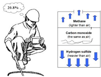
No tank is to be entered until the tank atmosphere has been thoroughly tested with approved and calibrated instruments. Following tests are to confirm that all areas of the tank, bottom in particular, are safe for entry, i.e.:
