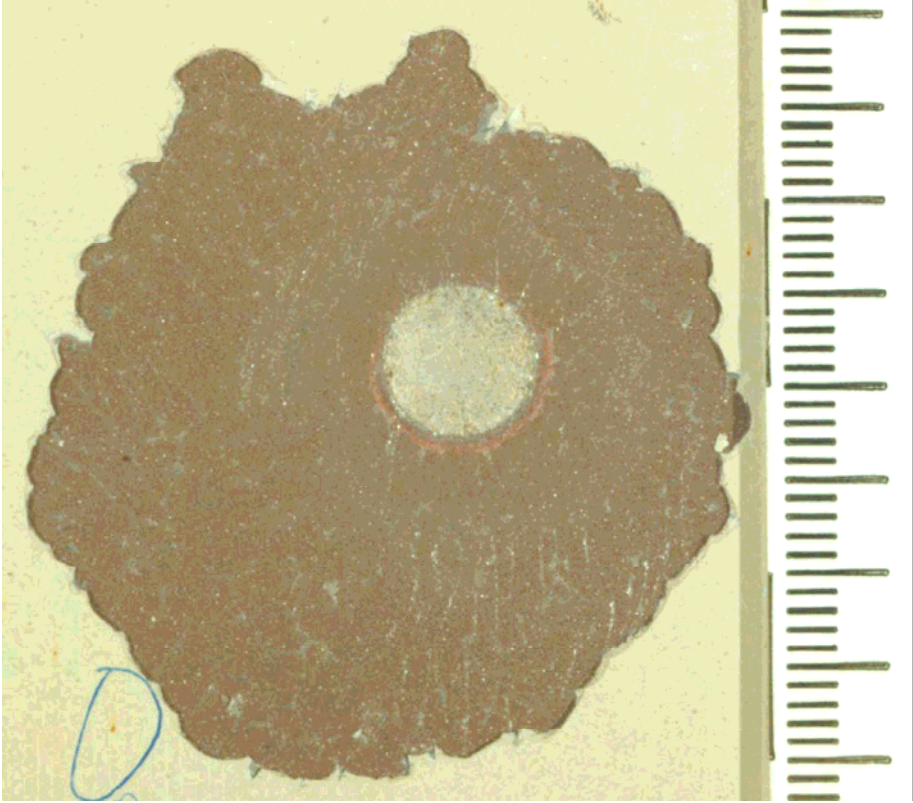
Figure C-7 Disbonding from artificial holiday, bottom wave tank panel (example picture not connected with example results in this model report).
