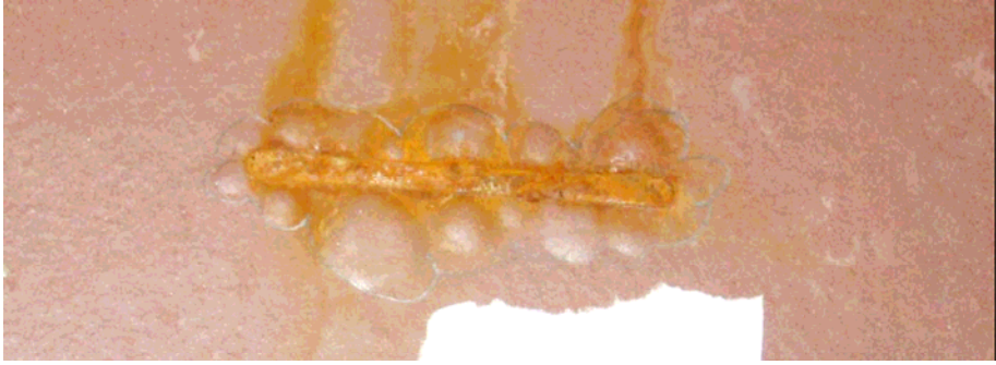
Figure C-3 Scribe area of top wave tank panel before removing of loose coating (example picture not connected with example results in this model report).
