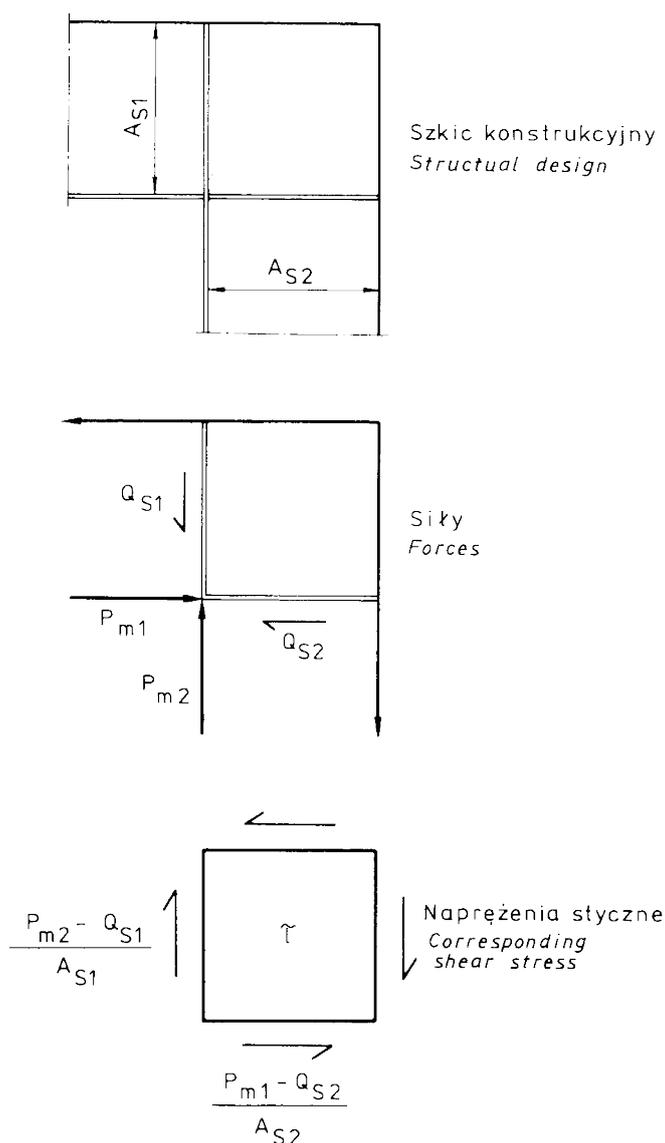
Fig.4.2-1 Stress analysis of cross joint
