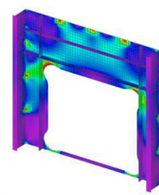
Fig. 5.2-4 An example of more dense FE mesh in the region of a window
