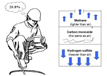
No tank is to be entered until the tank atmosphere has been thoroughly tested with approved and calibrated instruments. Following tests are to confirm that all areas of the tank, bottom in particular, are safe for entry, i.e.:
