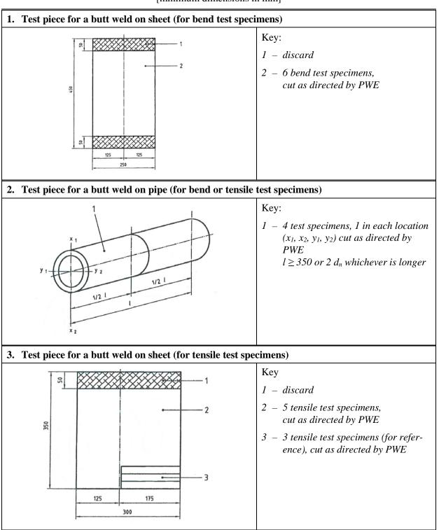
**Test pieces** [minimum dimensions in mm]
