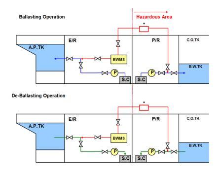
Appropriate Isolation Means: Two (2) screw down check valves in series with a spool piece or a liquid seal, or automatic double block and bleed valves
