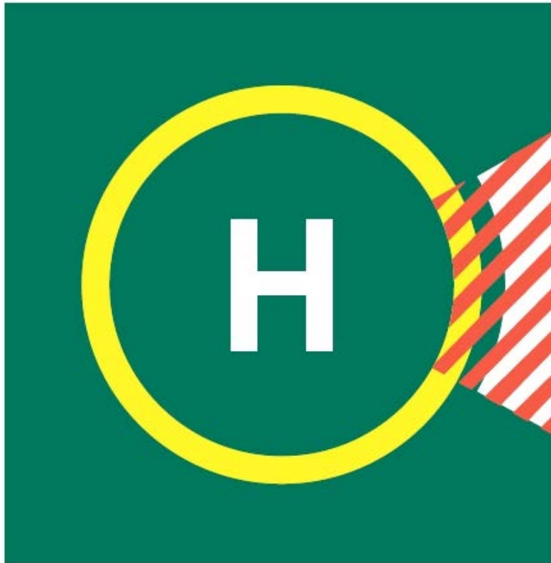
Fig. 5.6.3-2 Example of the mark of prohibited touch-down direction
