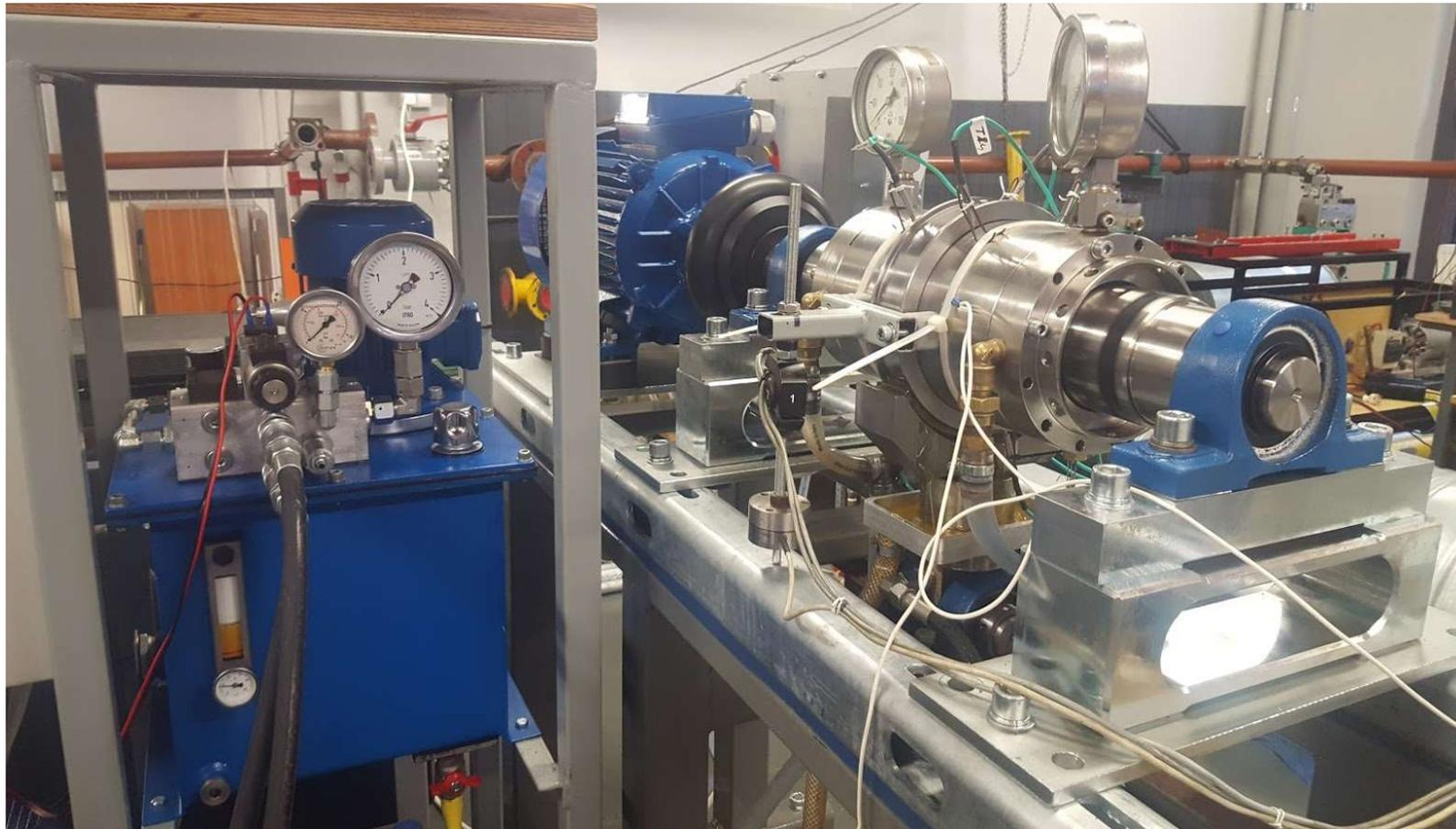
Water lubricated bearings test rig, with possibility of testing water / bio / water base liquids
