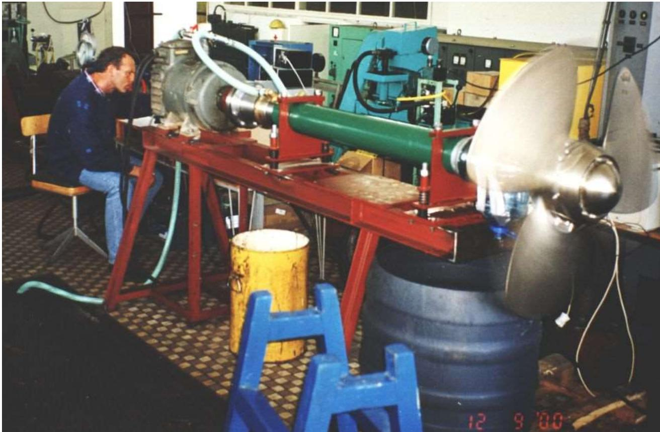
Experimental tests of water lubricated bearings with installation-ready propeller shaft and stern tube in 2000 – just before installation on small fishing vessel
