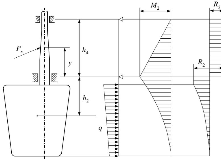
Fig. 3.2.3.3 Underhung rudder
