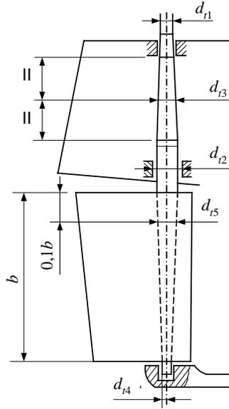
Fig. 3.4.1. Required rudder stock diameters
