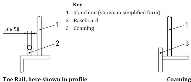
Fig. 11.1.1. Guard rails in way of deck edge
