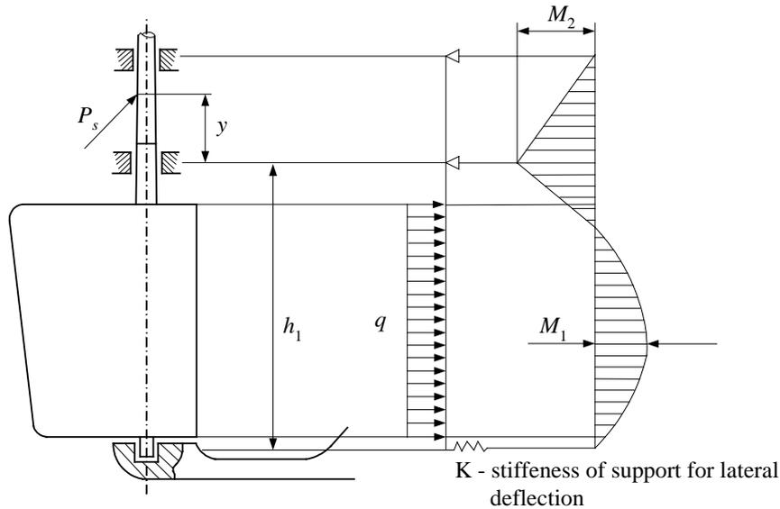
Fig. 3.2.3.2. Supported rudder
