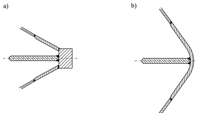
Fig. 3.8.1.1. Examples of suitable stems
