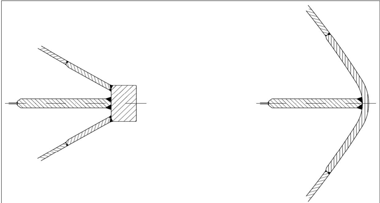
Figure 4-4. Examples of suitable stems.
