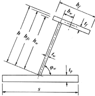
Figure 4 – Stiffener geometry
