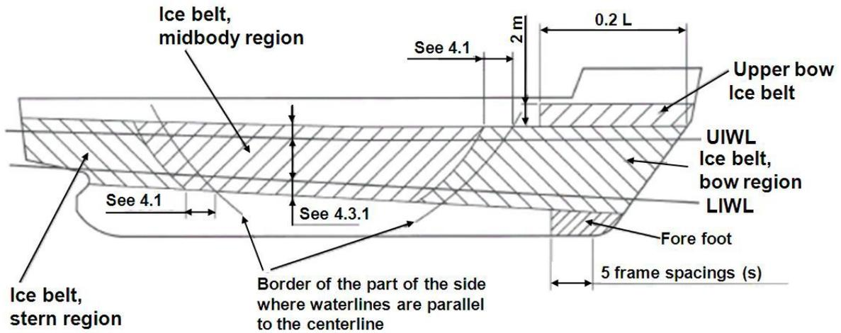
Figure 4-3. Ice strengthened regions of the hull
