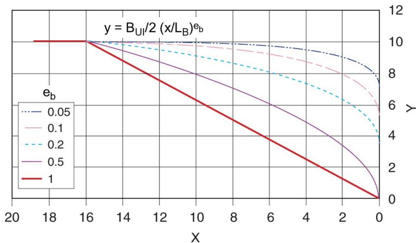
Figure 8 – Illustration of  $e_b$  effect on the bow shape for  $B_{\text{UI}} = 20$  and  $L_B = 16$
