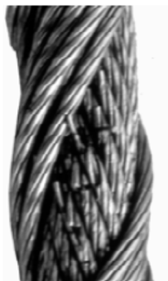
Fig. 7. Wire breaks in the internal layer of an ordinary lay rope, due to abrupt load – justification for immediate discard
