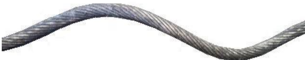
Fig. 8. Rope waviness (the longitudinal axis of the rope takes the shape of a helix). If the deformation exceeds the value indicated in 3.10 – the rope shall be discarded.
