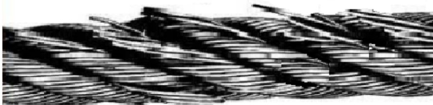
Fig. 1. Wire breaks and wire displacement over two adjacent strands in an ordinary lay rope – justification for discard.
