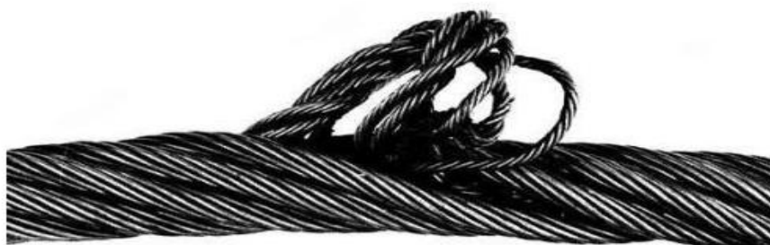
Fig. 10. Extrusion of a steel core, generally associated with a basket deformation (bird cage) – justification for immediate discard.
