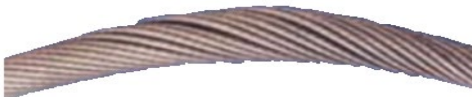
Fig. 11. One strand only affected by wire extrusion, examination over a length of rope shows that deformation is visible at regular intervals, normally of one lay length.
