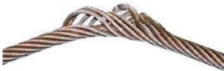
Fig. 9. Basket deformation (bird cage) – deformation of a multi-strand construction – justification for immediate discard.
