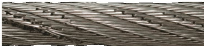
Fig. 6. Wire breaks in two strands, local to a compensating pulley, caused by jamming of the pulley – justification for immediate discard.
