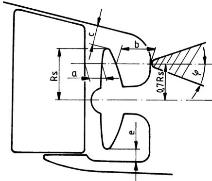
Fig. 11.4.2 Propeller clearance
