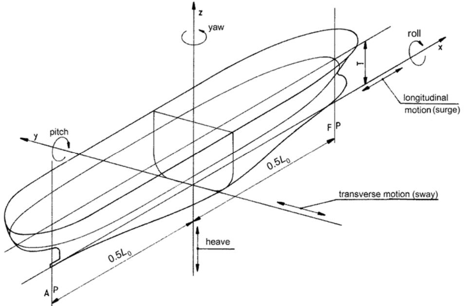
Fig. 17.5.2.1 Definition of Co-ordinate System and Ship motions
