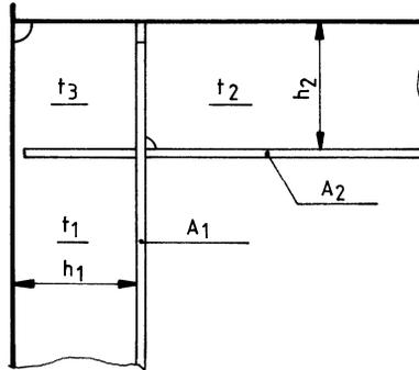
Fig. 13.8.3.5 Bracketless connection of girders
