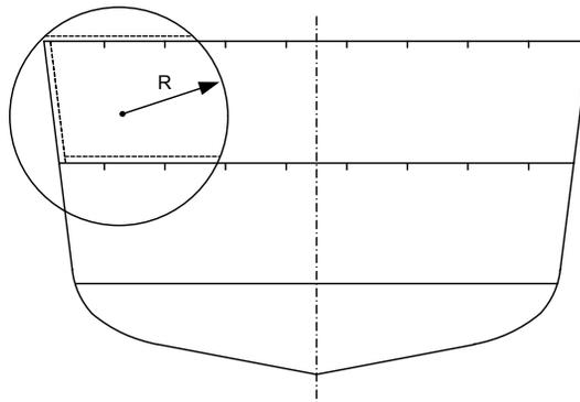
Fig. 6.2.1 The hull damaged region due to projectile explosion inside the ship
