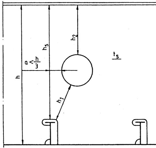
Fig. 3.2.3 Determining the net web height
