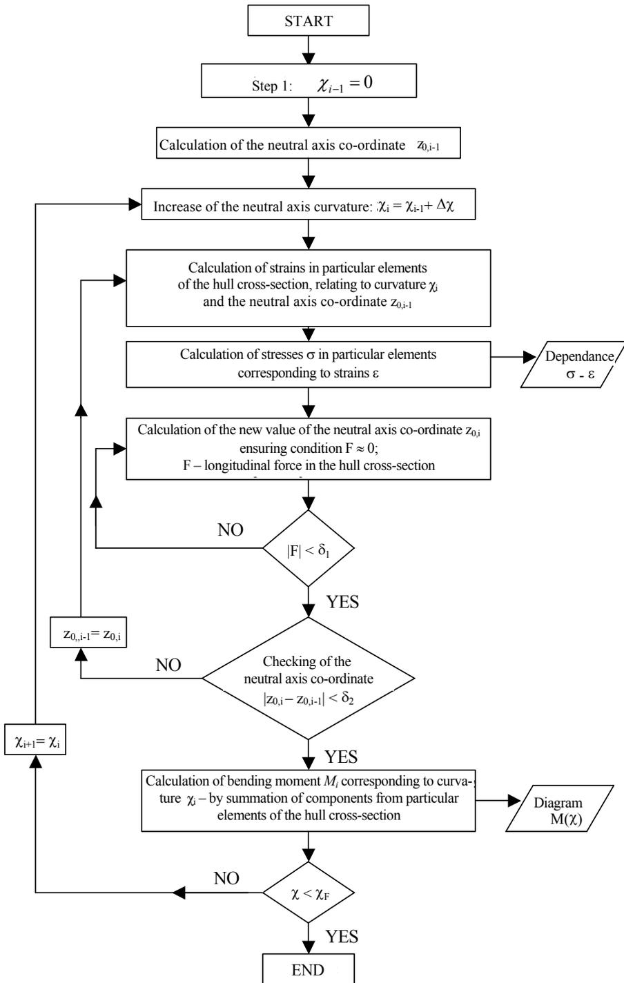
Fig. 2.1.1 Procedure for determination of  $M(\chi)$  dependence
