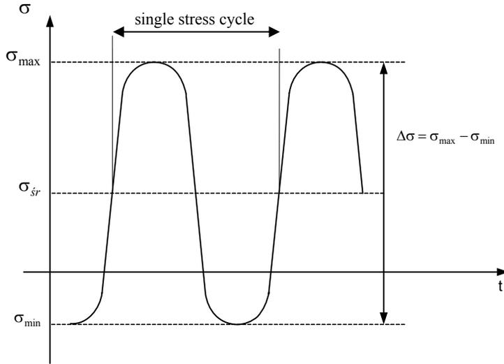
Fig. 16.2.3 Definition of stresses cycle and the range of stresses
