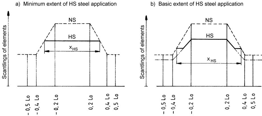
Fig. 15.6.2 Longitudinal extent of HS steel
