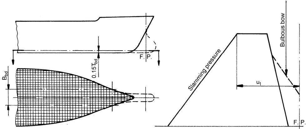
Fig. 6.7.5 Distribution of slamming pressure acting on the bottom
