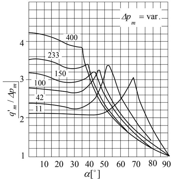
Fig. 4.2.3.1 Dependence  $q'_m / \Delta p = f(\alpha)$  for various values  $\Delta p_m$ .
