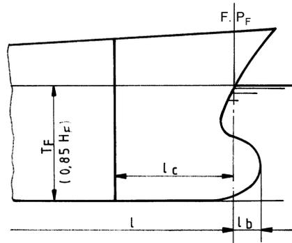
Fig. 9.2.2.1 Position of collision bulkhead
