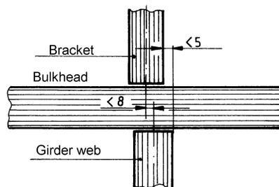
Fig. 4.2.3.5 Shift of interrupted planes
