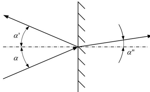
Fig. 4.3.4.1 Reflection and refraction of the underwater shock wave on the media border
