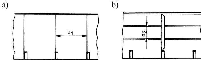
Fig. 3.6.3.1 Methods of stiffening the girder web
