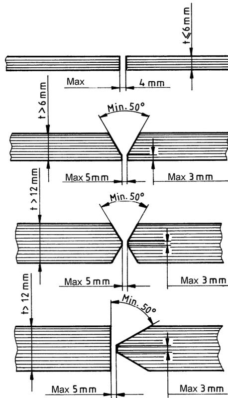
Fig. 4.2.1.1 Edge preparation for manual butt welding
