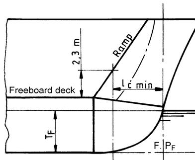
Fig. 9.2.2.3 Collision bulkhead with a ramp
