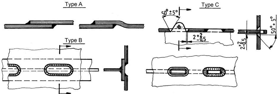
Fig. 4.2.2.1 Lap and slot welds
