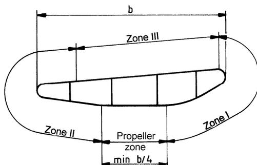
Fig. 11.5.2.1 Longitudinal section through nozzle ring
