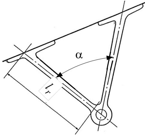
Fig. 11.6.3.8 Double-arm strut
