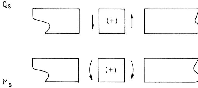
Fig. 15.4.2 Positive sense of bending moments and shear forces
