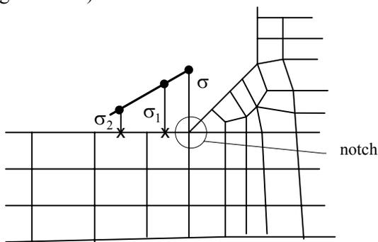
Fig. 14.7.5.1 Principle of stresses values extrapolation
