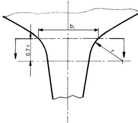
Fig. 11.3.6 Transition zone between rudder horn and hull plating
