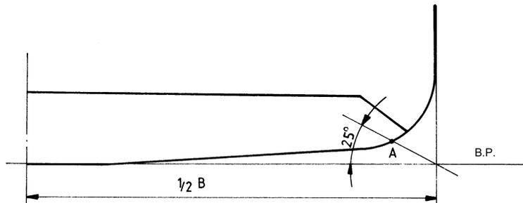
Fig. 6.1.2.4 Overlapping the bilge by the margin plate
