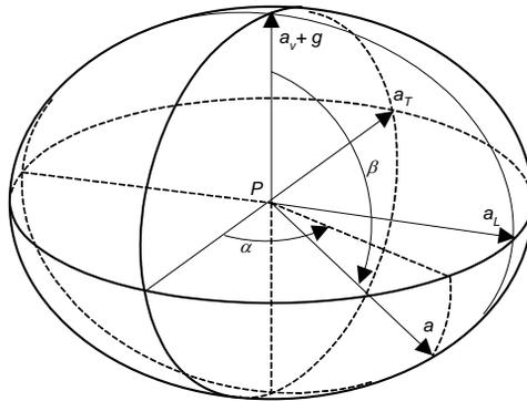
Fig. 17.5.4.4 Determining acceleration  $a$  of the ship's point  $P$  in any direction
