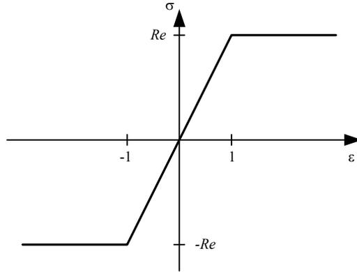
Fig. 2.2.3 Dependence  $\sigma - \varepsilon$  for elastic-plastic strains
