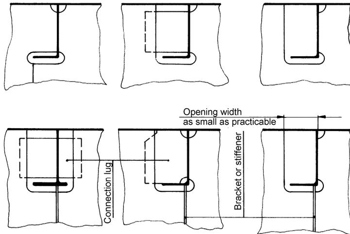
Fig. 4.3.7 Connection of a stiffener to the web plate of a girder
