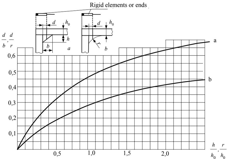
Fig. 14.3.2.7 Determination of rigid elements or rigid ends length
