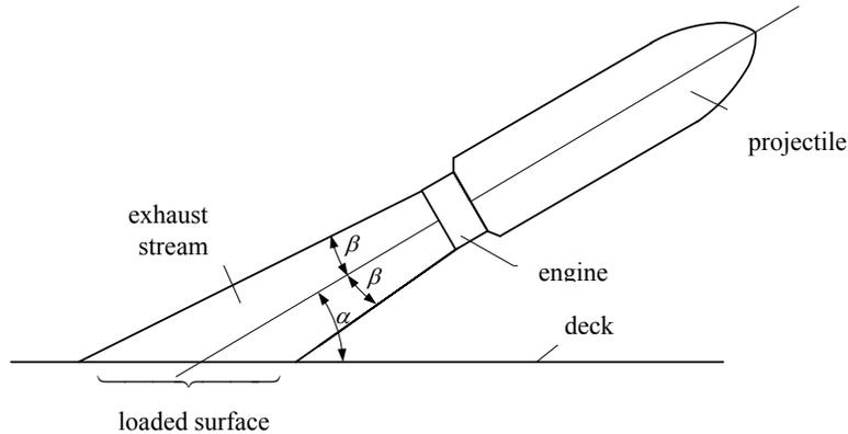
Fig. 5.4.1 Load from the exhaust stream
