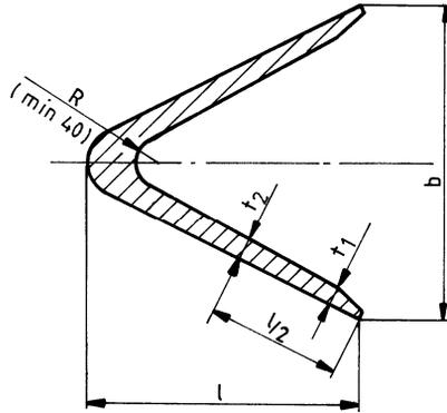
Fig. 11.7.2.4 Cast sternframe propeller post
