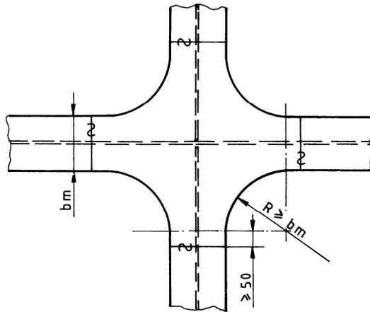
Fig. 3.3.2 Joints of girder face plates
