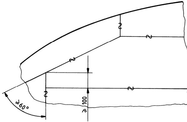
Fig. 3.3.1 Arrangement of welded joints
