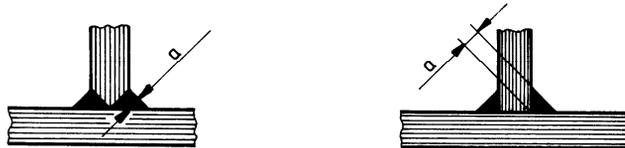
f) Thickness a of fillet weld
