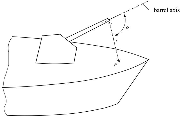
Fig. 5.3.3 Parameters for pressure  $p_z$  calculations
