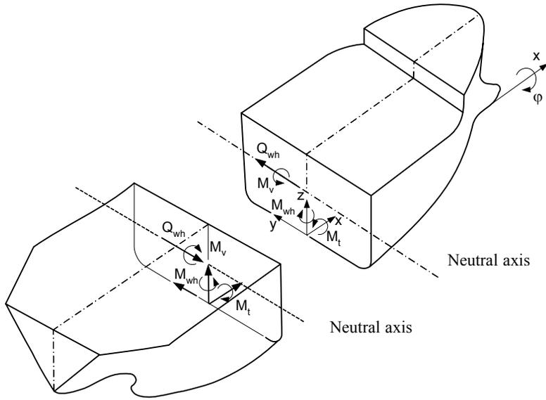
Fig. 15.13.3.5 Positive senses of the internal forces in the hull
