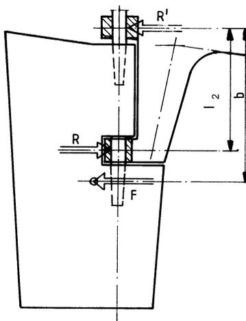
Fig. 11.3.2-2 Forces in semi-spade rudder
