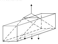
Fig. 3.2.2.4. Lifting from the bottom corner fittings
