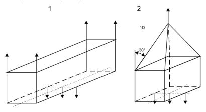
Fig. 3.2.2.3. Lifting from the top corner fittings
