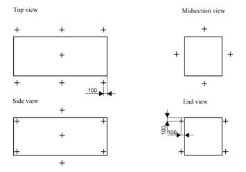
Fig. 3.5.3-2. Air temperature measurement points outside the container
