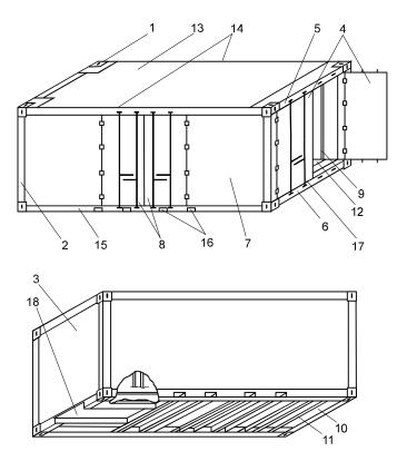
Fig. 1.2. Structural elements of a container (general purpose)
