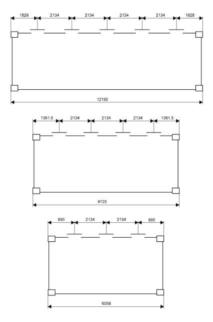
Fig. 2.5.1. Examples of the arrangement of openings for loading dry bulk cargo in non-pressurized box type containers
