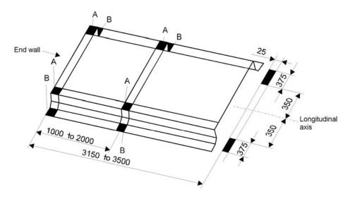
Fig. 3.3.4-2. Distribution of the load transfer areas in gooseneck tunnel (where the areas are not continuous)
