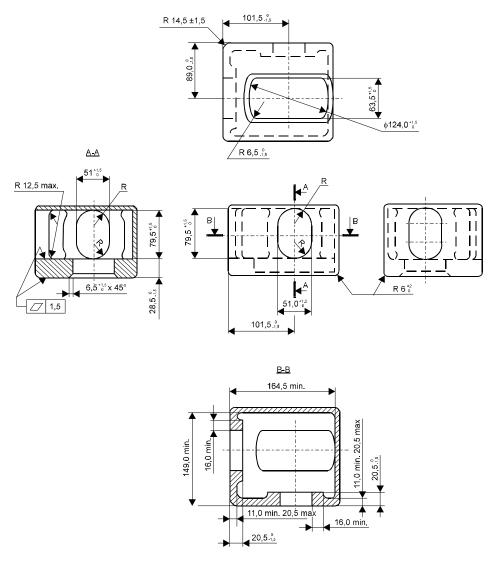
Fig. 3.2.1.1-3. Bottom corner fitting
