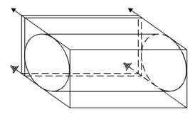
Fig. 3.5. Transverse strength test
