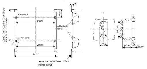
Fig. 2.9. Arrangement of intermediate sockets for clip-on units
