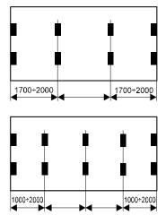
Fig. 3.3.6-4. Distribution of the load transfer areas in 1CC, 1C and 1CX containers
