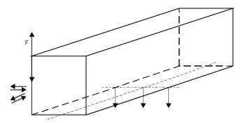
Fig. 3.3.2. Containers stacking strength test
