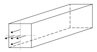
Fig. 3.8.1. End walls strength test
