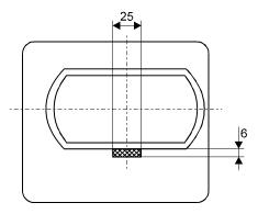
Fig. 3.2.1.3. Bottom corner fitting (bottom view)
