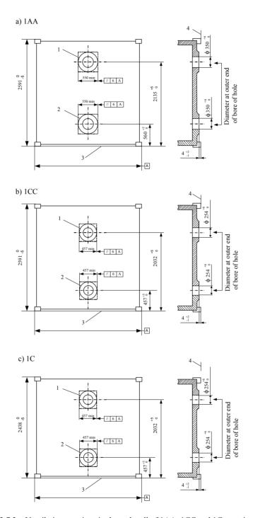
Fig. 2.7.2. Ventilation openings in the end wall of 1AA, 1CC and 1C containers
